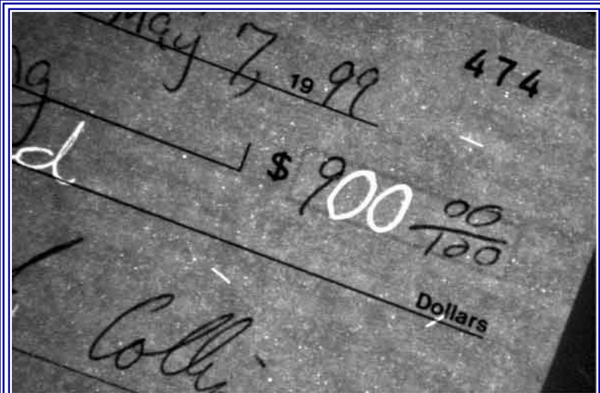
Image of a check with numbers fraudulently added to increase its value. The ink used to write the two zeros in the number "900" is different than the one used to write the remaining entries as revealed through IR luminescence and the VSC2000's integration feature.
